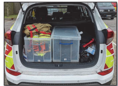
Figure 35: PPE with visible soiling, or the smell of smoke, should be bagged or stored in an airtight container.
