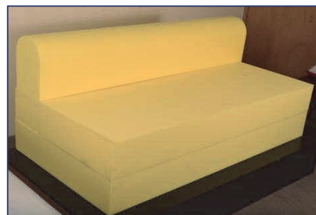
Figure 6: Polyurethane foam containing halogenated flame retardants (TCPP)
